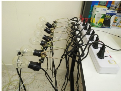
Figure 3.9 Six 100W incandescent lamps
