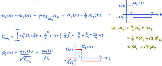
iii. Find the two vectors,  $\vec{\mathbf{s}}^{(1)}$  and  $\vec{\mathbf{s}}^{(2)}$ , that represent the two waveforms  $s_1(t)$  and  $s_2(t)$  in the new axes based on  $\phi_1(t)$  and  $\phi_2(t)$ . Draw the corresponding constellation in the figure below.
