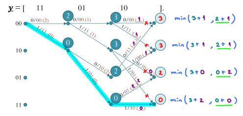
Suppose that we observe  $\underline{v}$  = [110110] at the input of the minimum distance decoder. Apply Viterbi algorithm to find the decoded codeword  $\hat{\underline{x}}$  and the decoded message  $\hat{\mathbf{b}}$ .
