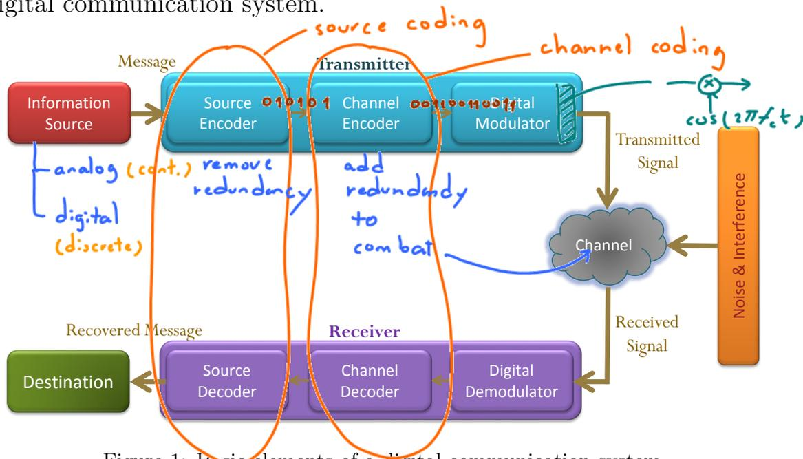
Figure 1: Basic elements of a digital communication system
