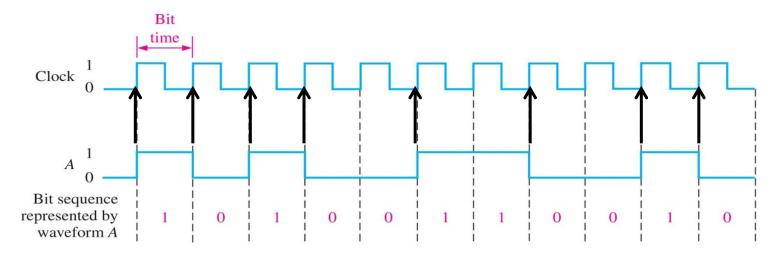
• Notice that change in level of waveform *A* occurs at the leading edge of the clock waveform.
