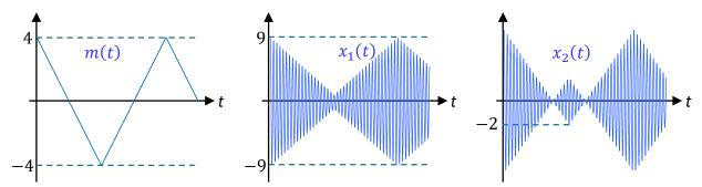
The middle and the rightmost plots show two AM signals  $x_1(t)$  and  $x_2(t)$  produced by using two different values of modulation index. During the previous in-class exercise, we have calculated the values of A and  $\mu$ . They are summarized in the table below.
