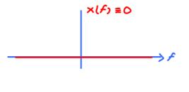
c. Plot X(f) when the frequency response of the BPF is  $H(f) = \begin{cases} 4, & |f - 150| \le 5, \text{ 145} \le f \le 155 \\ 4, & |f + 150| \le 5, \text{ -155} \le f \le -145 \end{cases}$  0, otherwise.
