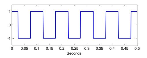
(b)  $sgn(cos\omega_0 t) = 2 \times 1[cos\omega_0 t \ge 0] - 1$ . So, a = 2 and b = -1.
