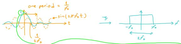
Then, we draw the sinc (27 fot) using the zeroes of sin (27 fot) We then see that the first zero occurs at 1/27. Therefore, in the freq. domain, the corresponding rectangular function has width = 2 %. So, its boundaries are ± %. Conclusion: sinc (27 fot) is bandlimited to B = fo Note that the height of the rectangular function must be 1 to make its area = 1.
