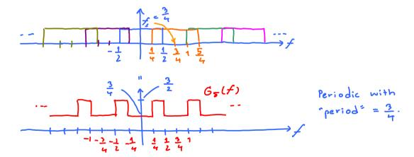
With  $T_s = 1$ ,  $g[n] = g(nT_s) = g(n \times 1) = g(n) = sinc(\pi n)$ . (d.i) From the plot of  $sinc(\pi n)$  drawn earlier, we have  $g[n] = \begin{cases} 1, & n = 0, \\ 0, & \text{other wise}. \end{cases}$
