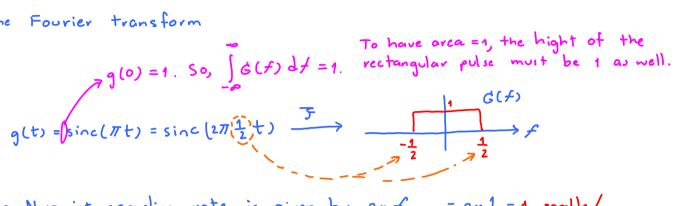
(b) The Nyquist sampling rate is given by  $2 \times f_{max} = 2 \times \frac{1}{2} = 1$  sample/sec.
