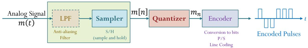
Figure 71: PCM System Diagram
