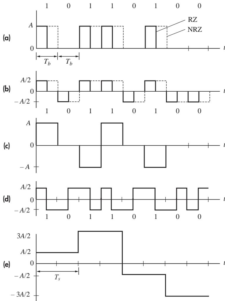
Figure 75: Line codes with rectangular pulses: (a) unipolar RZ and NRZ; (b) polar RZ and NRZ; (c) bipolar NRZ; (d) split-phase Manchester; (e) polar quaternary NRZ. [3, Fig 11.1-1 p 483]
