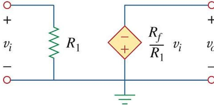
The voltage gain is  $A_v = v_o/v_i = -R_f/R_1$ .
