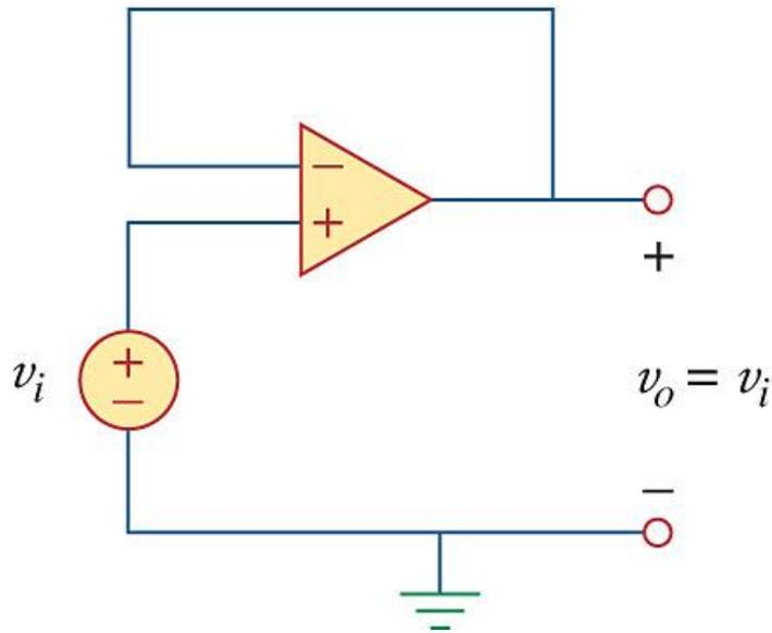
A voltage follower is used to isolate two cascaded stages of a circuit.
