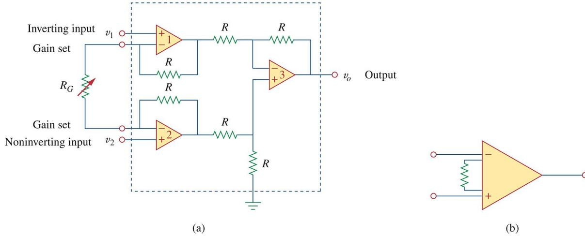
$$v_0 = \left( 1 + \frac{2R}{R_G} \right) (v_2 - v_1).$$
