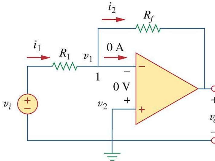
The equivalent circuit for the inverting amplifier is:
