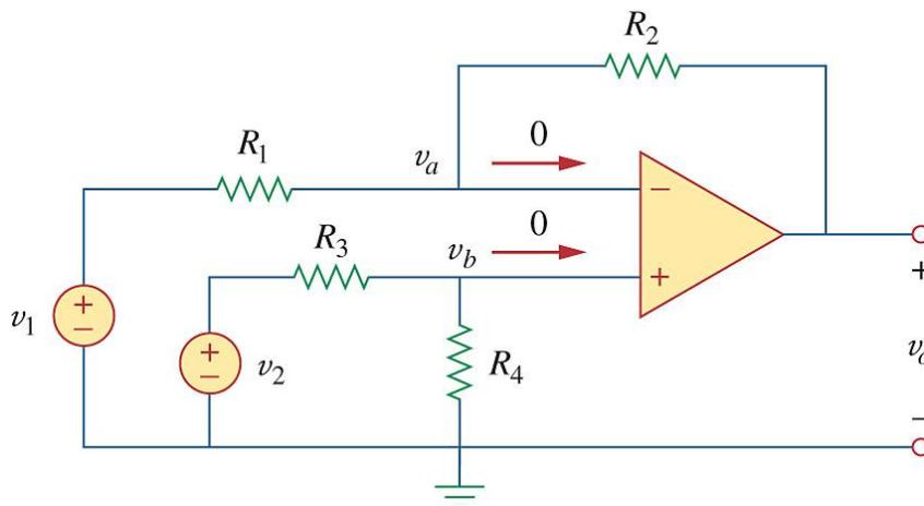
$$v_o = \frac{R_2(1 + R_1/R_2)}{R_1(1 + R_3/R_4)}v_2 - \frac{R_2}{R_1}v_1$$
