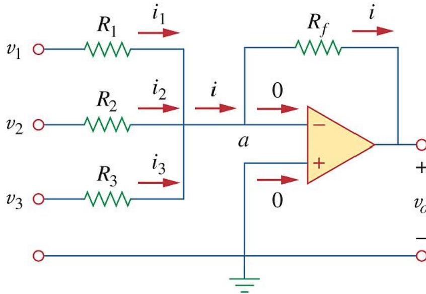
$$v_o = - \left( \frac{R_f}{R_1} v_1 + \frac{R_f}{R_2} v_2 + \frac{R_f}{R_3} v_3 \right).$$
