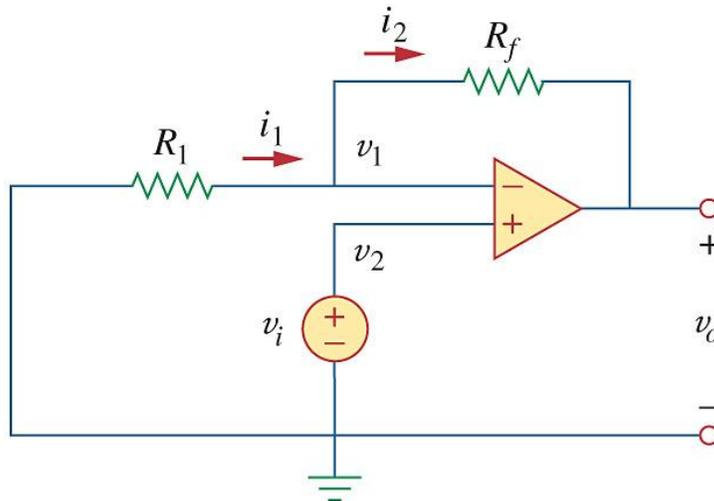
The voltage gain is  $A_v = \frac{v_o}{v_i} = 1 + \frac{R_f}{R_1}$ , which does not have a negative sign. Thus the output has the same polarity as the input.
