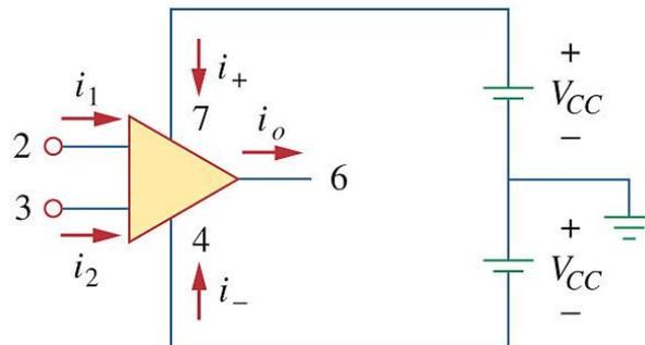
Although the power supplies are often ignored in op amp circuit diagrams for the sake of simplicity, the power supply currents must not be overlooked:
