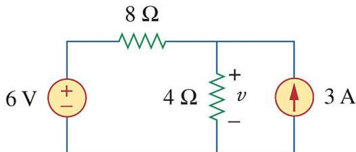
The **superposition principle** states that the voltage across (or current through) an element in a linear circuit is the algebraic sum of the voltages across (or currents through) that element due to each independent source acting alone.
