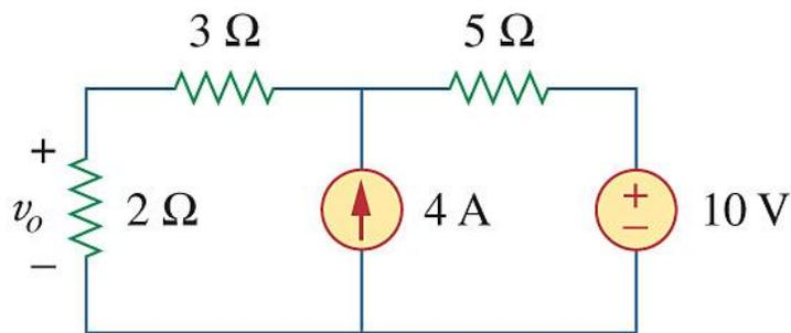
Remark: Superposition helps reduce a complex circuit to simpler circuits through replacement of voltage sources by short circuits and of current sources by open circuits.
