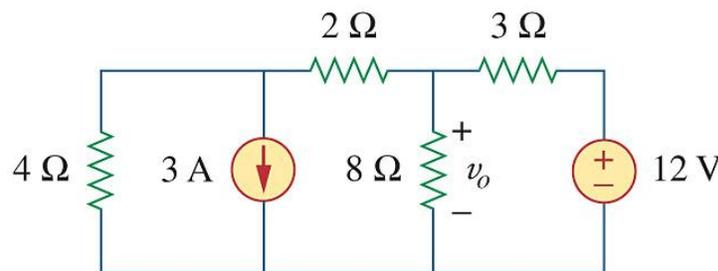
Remark: From (4.1), an ideal voltage source with  $R = 0$  cannot be replaced by a finite current source. Similarly, an ideal current source with  $R = \infty$  cannot be replaced by a finite voltage source.
