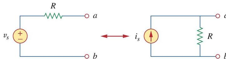
Notice that when terminals  $a - b$  are short-circuited, the short-circuit current flowing from  $a$  to  $b$  is  $i_{sc} = v_s/R$  in the circuit on the left-hand side and  $i_{sc} = i_s$  for the circuit on the righthand side. Thus,  $v_s/R = i_s$  in order for the two circuits to be equivalent. Hence, source transformation requires that
