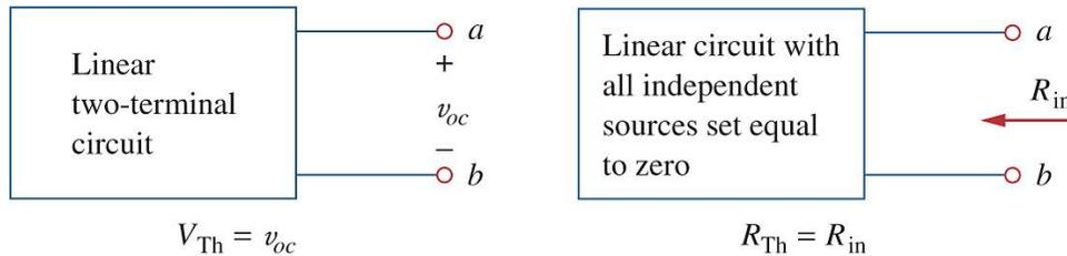
**S3:** Connect  $V_{TH}$  and  $R_{TH}$  in series to produce the Thevenin equivalent circuit for the original circuit.
