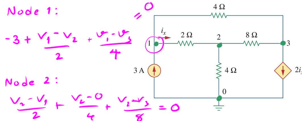
$$i_x = \frac{V_1 - V_2}{2}$$
