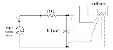
1) The plot below shows the voltage across the generator. On the same plot, sketch the voltage across the capacitor.
