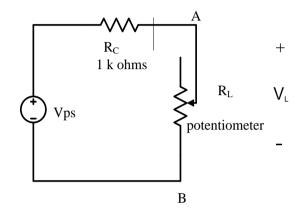
Figure 3-4: A circuit for verifying the maximum power transfer condition.
