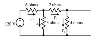
**Figure 3-1**(b): Circuit in Figure 3-1(a) with the current source deactivated (replaced by an open circuit).
