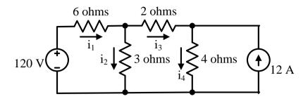
**Figure 3-1**(a): Circuit to illustrate superposition technique.
