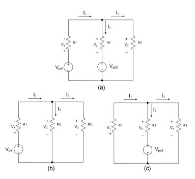
**Figure 3-5:** Circuits to verify superposition theorem in lab 03: (a) original circuit, (b) modified circuit with  $V_{ps1}$  only, and (c) modified circuit with  $V_{ps2}$  only.
