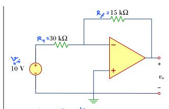
$$V_{0} = -\frac{R_{f}}{R_{1}}V_{2} = -\frac{45h}{26h} \times 10^{5} = -5 \text{ } \checkmark$$
