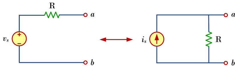
Notice that when terminals  $a - b$  are short-circuited, the short-circuit current flowing from  $a$  to  $b$  is  $i_{sc} = v_s/R$  in the circuit on the left-hand side and  $i_{sc} = i_s$  for the circuit on the righthand side. Thus,  $v_s/R = i_s$  in order for the two circuits to be equivalent. Hence, source transformation requires that
