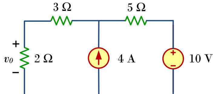
4.2.8. Remark on linearity: Keep in mind that superposition is based on linearity. Hence, we cannot find the total power from the power due to each source, because the power absorbed by a resistor depends on the square of the voltage or current and hence it is not linear (e.g. because  $5^2 \neq 1^2 + 4^2$ ).
