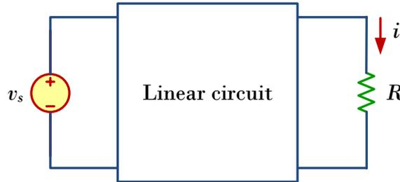
The circuit is terminated by a **load**  $R$ . We take the current  $i$  through  $R$  as the output. Suppose  $v_s = 10$  V gives  $i = 2$  A. By the assumed linearity,  $v_s = 1$  V will give  $i = 0.2$  A. By the same token,  $i = 1$  mA must be due to  $v_s = 5$  mV.
