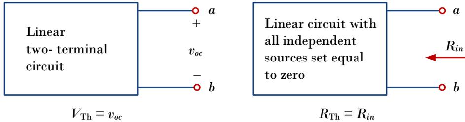
**S3:** Connect  $V_{Th}$  and  $R_{Th}$  in series to produce the Thevenin equivalent circuit for the original circuit.
