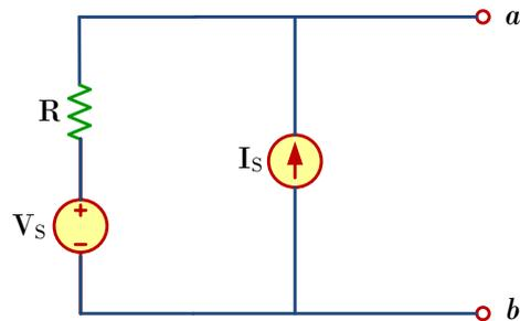
EXAMPLE 4.5.5. *Directly* find the Norton equivalent circuit of the circuit in the following figure at terminals a-b.
