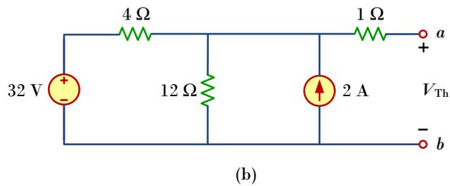
EXAMPLE 4.4.6. Determine the current  $I$  in the branch a-b in the circuit below.
