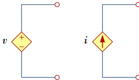
1.3.4. The key idea to keep in mind is that a voltage source comes with polarities (+ -) in its symbol, while a current source comes with an arrow, irrespective of what it depends on.
