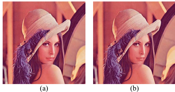
Figure 4. Quantization of the image "Lena". (a) The original image and (b) the 256-color quantized image of the proposed algorithm.
